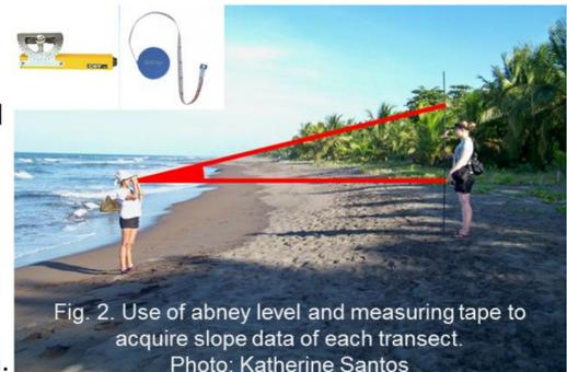
Fig. 2. Use of abney level and measuring tape to acquire slope data of each transect. Photo: Katherine Santos
